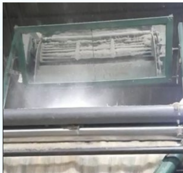
Figure 9: Generation of floating dust during carding
