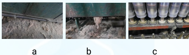
Figure 6: Generation of caddis during (a) breaker carding (b) finisher carding (c) spinning
