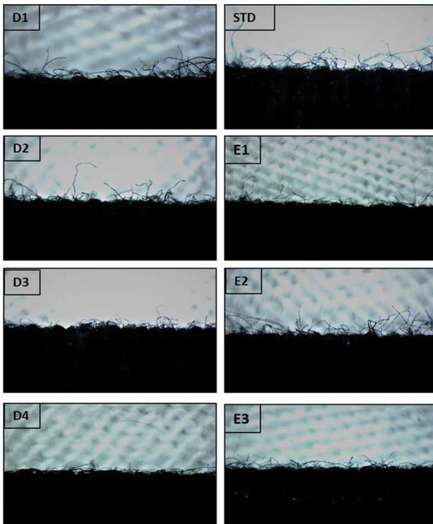
Figure 10: Surface view for samples treated with Acid cellulase and Bio polish enzyme -880 at different concentrations
