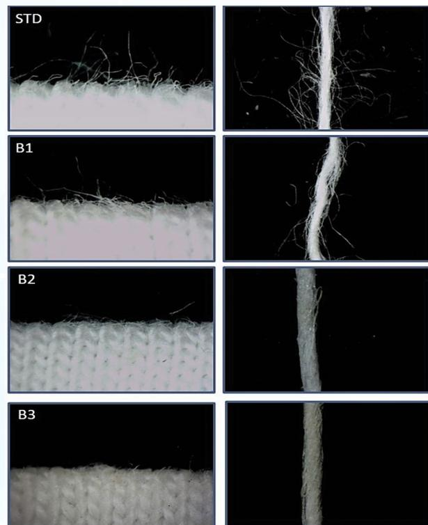
Figure 8: Surface view of samples treated with Biopolish enzyme-880 at different concentrations
