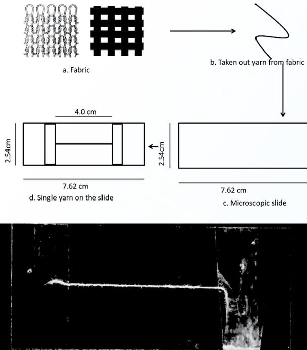
Figure 6: Experimental design for surface analysis (for yarn)
