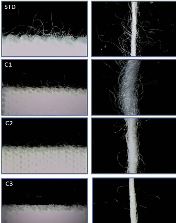
Figure 9: Surface view of samples treated with Azypolish-AC enzyme at different concentrations
