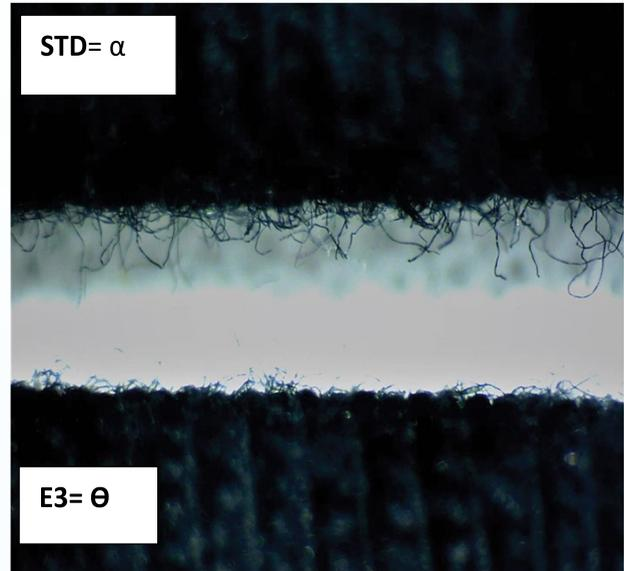
Figure 11: Comparative view of samples of STD and 3% ENZ cellulase enzyme
