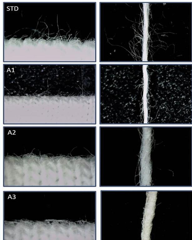
Figure 7: Surface view of samples treated with ENZ cellulase enzyme at different concentrations
