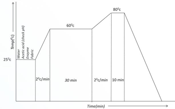
Figure 4: Process curve of biopolishing
